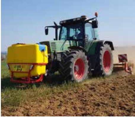
LF 600 M1 combined with a rotary harrow or tiller for application of soil-strengthening microorganisms in organic farming
