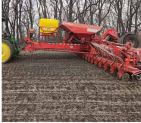
LF 600 M1 combined with a grain seeder for application of liquid fertilizer during seeding
