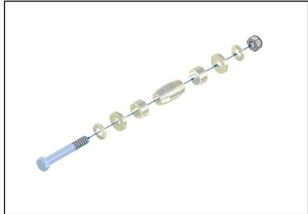
Figure 7: structure of the clamping bolt
