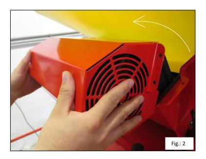
3. Take the top part of the straw protection cover in your hand and attach it to the steel frame on both sides with the previously loosened screws.
