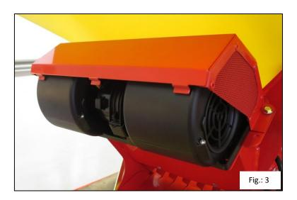
4. Now attach the bottom part of the straw protection cover by threading the 3 elongated slots, located on the top side of this part, upwards into the hooks that can be seen in Fig. 3.
