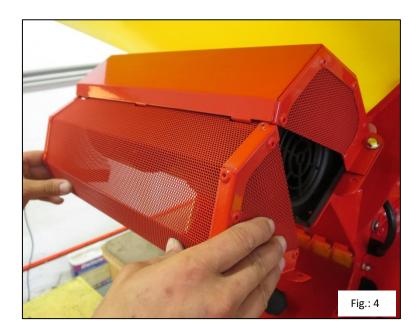
5. Position the second part of the straw protection cover on the steel frame such that the drilled holes of the straw protection cover overlap with those of the steel frame. Attach this part onto the steel frame with the previously loosened screws.
